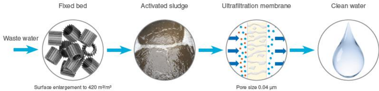
Illustration 5: Unique plant combination (anaerobic pretreatment combined with an MBR plant)
